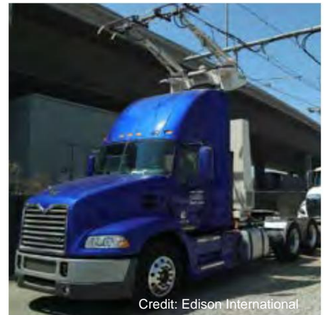
Figure 3-1: Vehicles and overhead line charging for a pilot project in California
